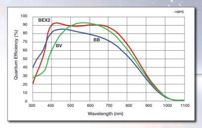
A range of sensor options are available for the iKon-XL 231 that provide high photon collection efficiency for maximising the SNR. Deep depletion (-DD) sensor options provide extended NIR sensitivity.
