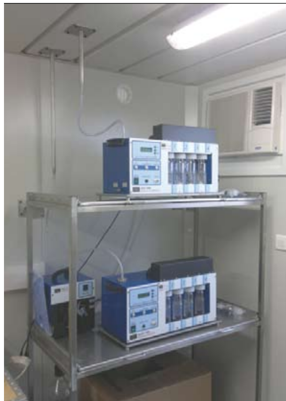
MARC 7000 tritium and HAGUE 7000 carbone 14 samplers installed on a stainless steel shelf, with atmospheric sampling probes.
