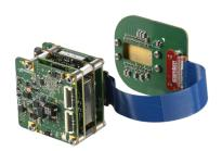
C-RED New Space is a SWIR camera core specifically tailored for satellite optical payloads. Based on a VGA InGaAs sensor with a resolution of 640x512 pixels and a 15  $\mu$ m pixel pitch, the camera is sensitive in the 0.9 to 1.7  $\mu$ m range with a quantum efficiency exceeding 70% from 1000 to 1650 nm.
