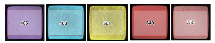
A series of intensity maps captured at the exit window of Dragonfly across all major wavelengths from 405 nm to 750 nm. A high degree of uniformity is visible. This uniformity then translates to the sample with high quality chromatically corrected objectives in the microscope.
