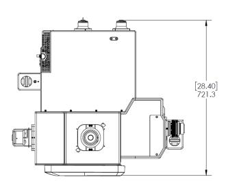
Note: Shown without installation handles, depth is 30.7 [780] with handles. For dimensions of the ILE, please refer to the <u>ILE</u> specifications sheet.
