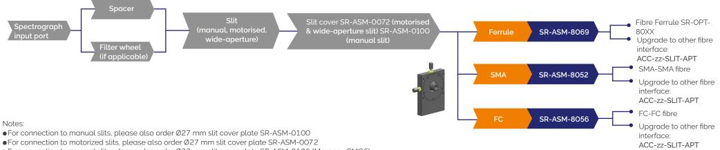
• For connection to manual slits, please also order Ø32 mm slit cover plate SR-ASM-0106 (Marana sCMOS) • For connection to motorized slits, please also order Ø32 mm slit cover plate SR-ASM-0107 (Marana sCMOS)
