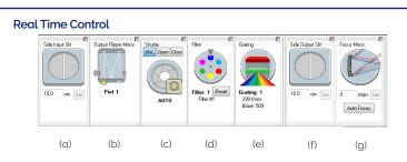
(a and f) Slit drive: Control the spectrograph slit width - drag blades on icon or type in required slit width
