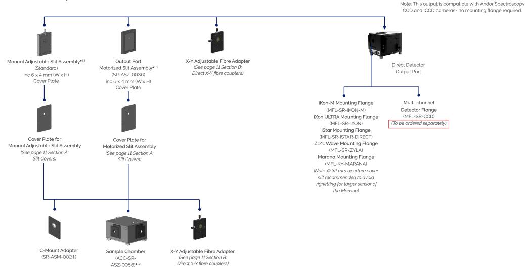
Note: a flange MUST be ordered separately for any configuration involving a multichannel or InGaAs detector.
