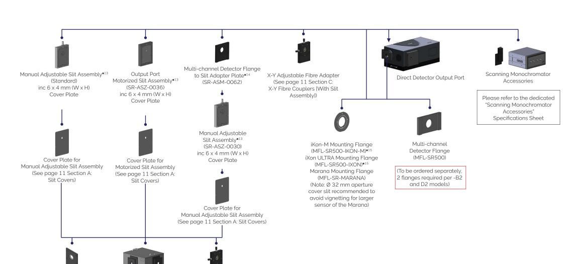
Note: a flange MUST be ordered separately for any configuration involving a multichannel or InGaAs detector.
