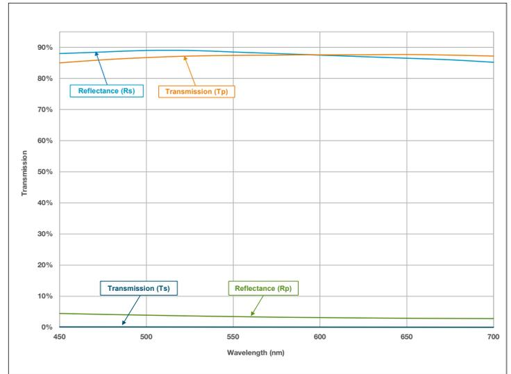
The graphs above show the transmission and reflectance curves for Semrock imaging dichroic beamsplitters and Moxtek optically flat polarizing beamsplitters. Both types of beamsplitter are optimized for use at a 45° angle of incidence.
