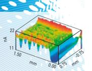
The 3300 bi-potentiostat/FRA can make low current, low noise measurements simultaneously at the tip and substrate to address specialist applications in surface science and the study of living cells. ac-SECM is a new technique that has the capability to measure surface phenomena without the presence of a mediator. This feature is useful in the field of corrosion as it allows measurement without the need for additional chemicals.
