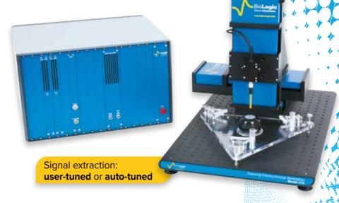
The surface work function can be directly correlated to many aspects of surface condition including corrosion potential. Moreover, as the technique utilises a capacitance probe, it can be used to measure the topography of the sample.
